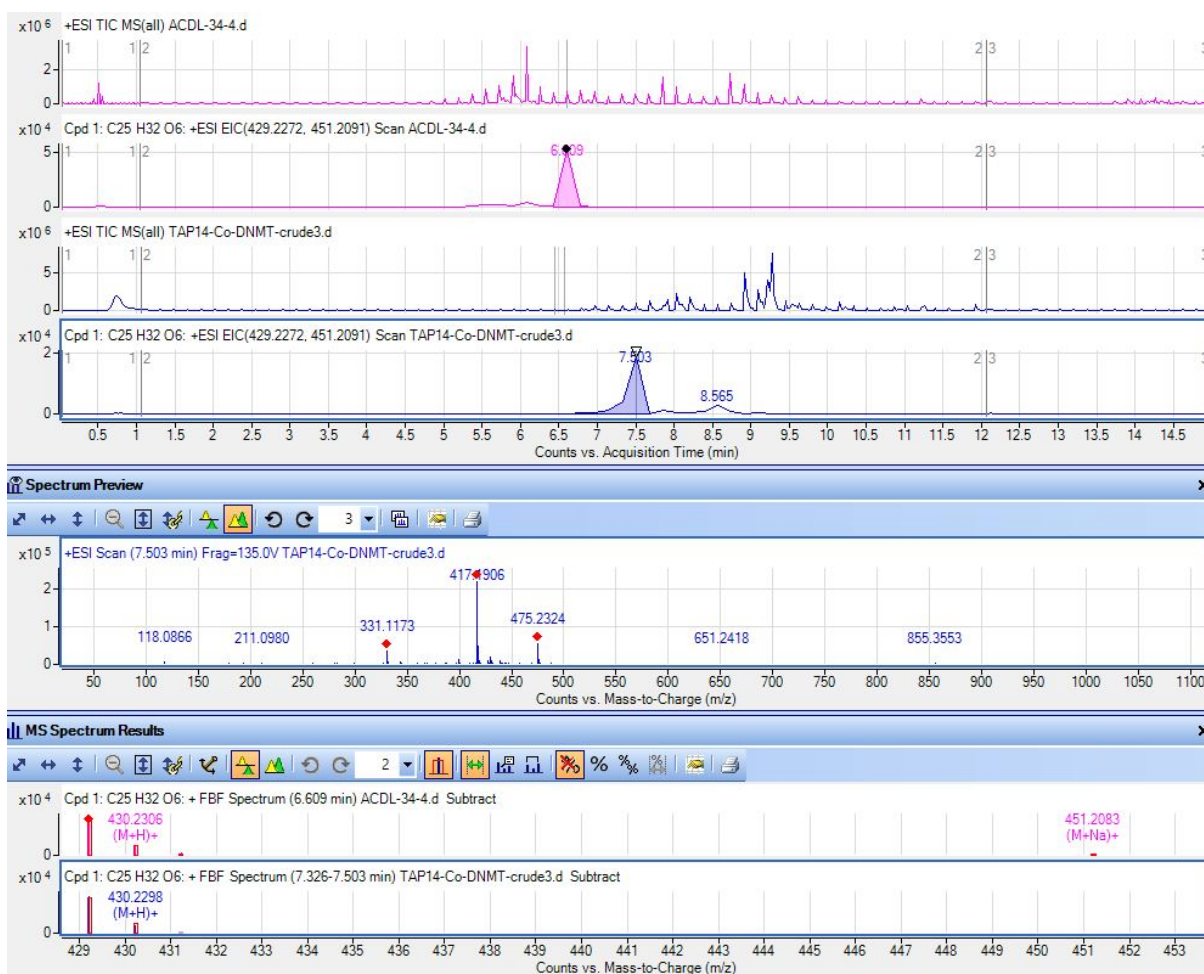
Figure V.4.2.3. MS/MS spectra for day 3 crude extract (black) prepared from co-culture and standard solution of tapachulanone A ( 13 ) (pink).
